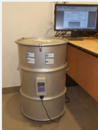
concrete calorimeter for Heat of Hydration
