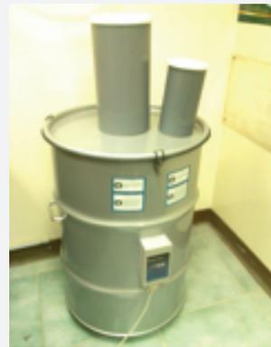
Figure 1: A simple and rapid test device for monitoring the heat of hydration of concrete mixtures for both laboratory and field applications
